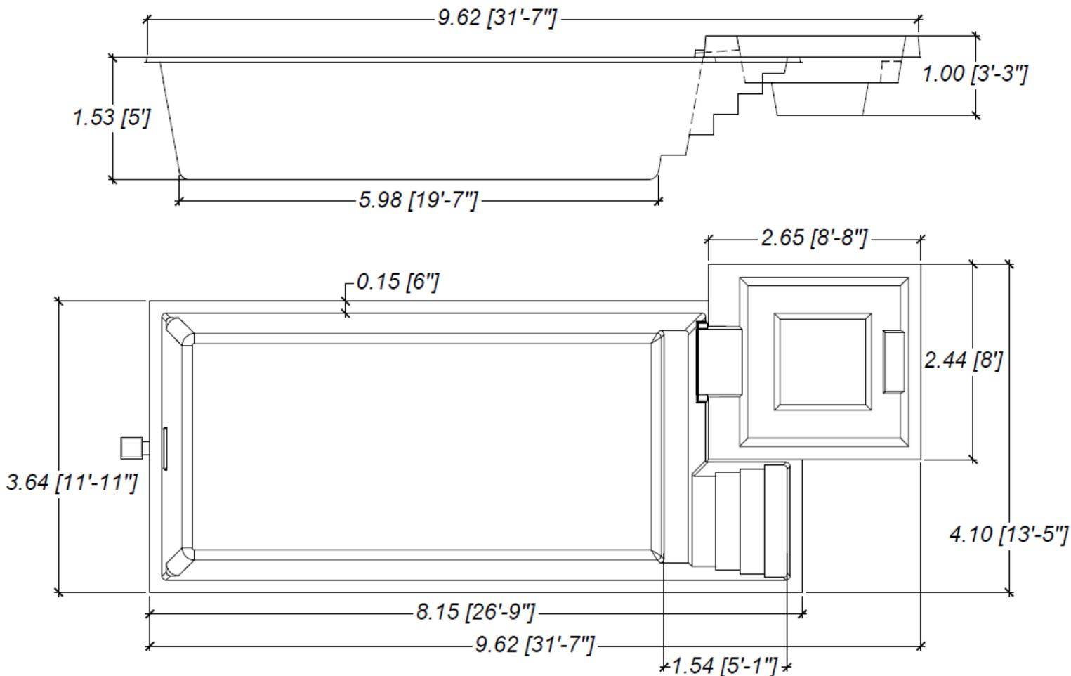
Structure de la piscine entièrement en fibre de verre. / Structure of the swimming pool entirely in fiberglass.
